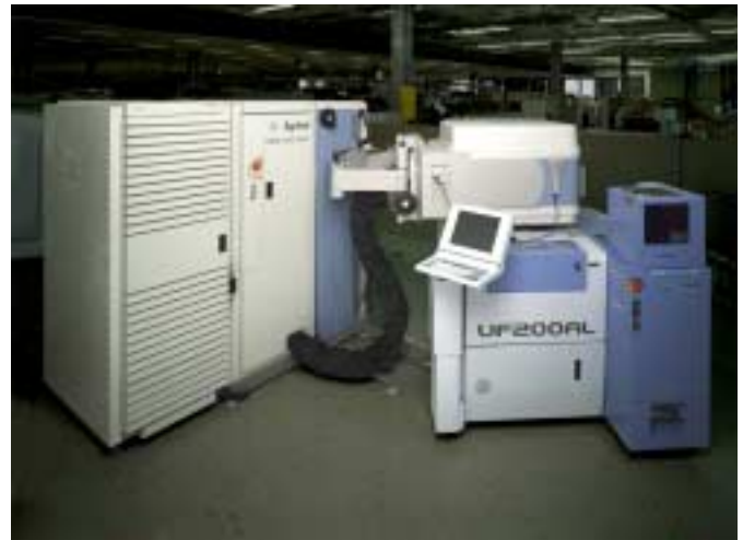
Figure 2. ATE used for on-wafer RF measurements (Agilent 93000 with RF Measurement Suite docked to a TSK wafer probe station).
